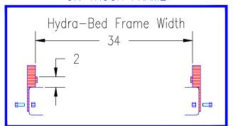
Bolt 2 1/2x2 1/2x54" tube to factory frame risers placing reinforcing plates under risers. Center Hydra-Bed 10" from each end of tube. Weld Hydra-Bed frame to tube risers. Hydra-Bed frame will be resting on tube and between risers.
